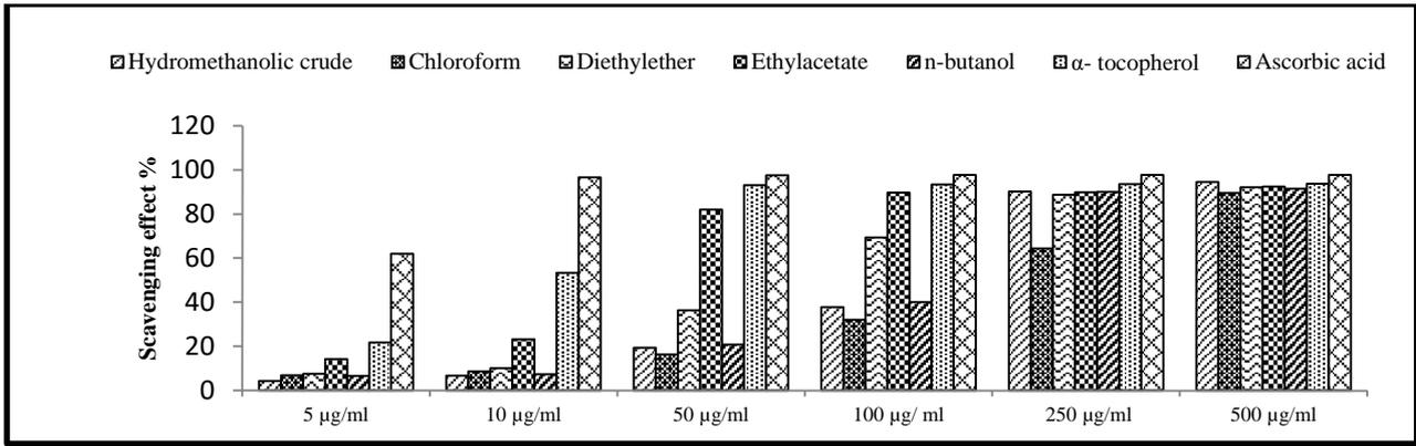
Figure 1: The DPPH radical scavenging activities of ascorbic acid, α-tocopherol and extracts of *A. graveolens*. Each value is expressed as mean ± SD (n = 3).
