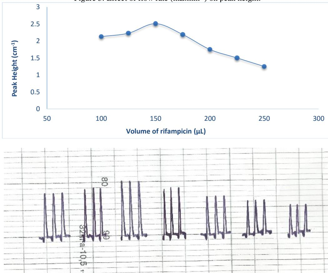
Figure 4: Effect of sample volume (µL) on peak height.
