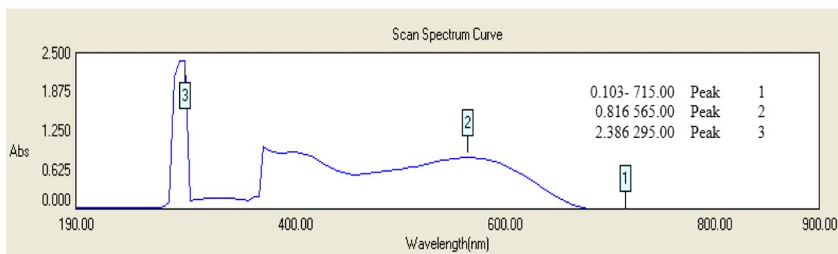
Figure 2: The UV-Visible spectrum of rifampicin –copper ion (II) complex.
