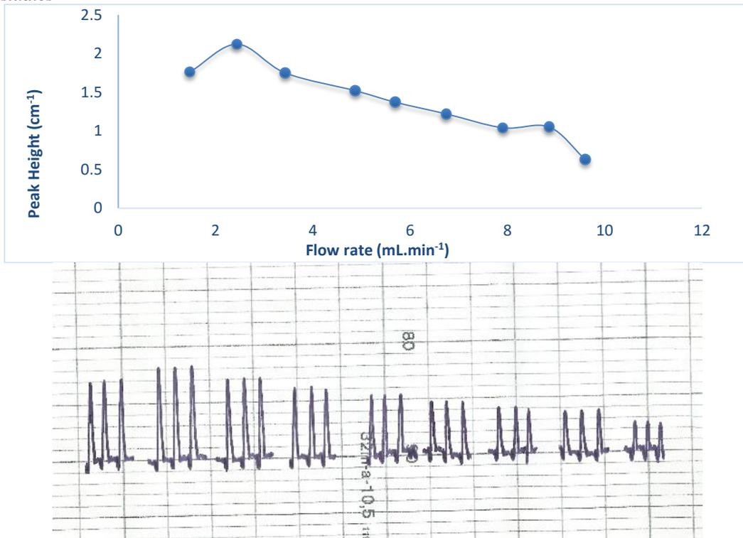
Figure 3: Effect of flow rate (mL.min<sup>-1</sup>) on peak height.
