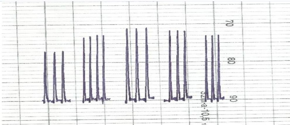
Figure 7: Effect of reaction coil length (cm) on peak height.
