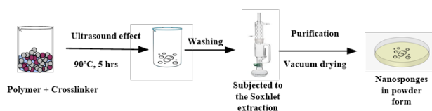
Figure 3: Ultrasound-assisted method for development of nanosponges
