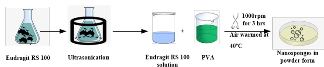
Figure 7: Quasi-emulsion solvent method
