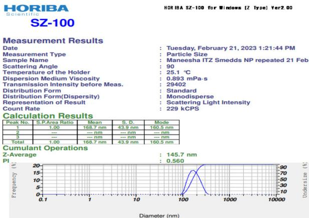
**Figure 4:** Globule size of optimised ITZ L-SMEDDS (ILS<sub>6</sub>)
