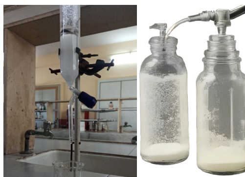
Figure 1: Extraction of allicin using a glass column for the separation and purification of allicin from fresh snow mountain garlic samples
