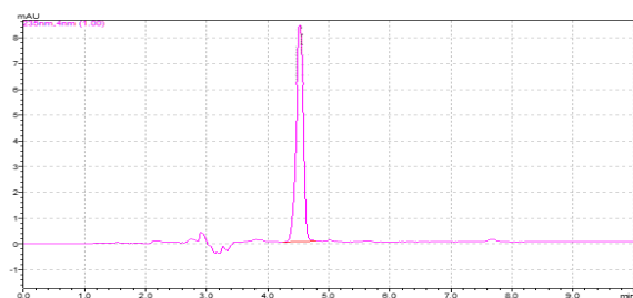
Figure 3: Trial chromatogram obtained by using MEOH: \text{KH}_2\text{PO}_4 Buffer (0.05M):(80:20 pH 5.5) as mobile phase
