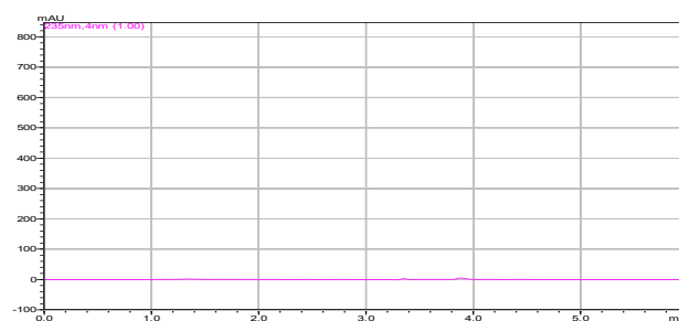
Figure 1: Blank chromatogram obtained by using MEOH: KH 2 PO 4 Buffer (0.05M):(65:35 pH 6.1) as mobile phase
