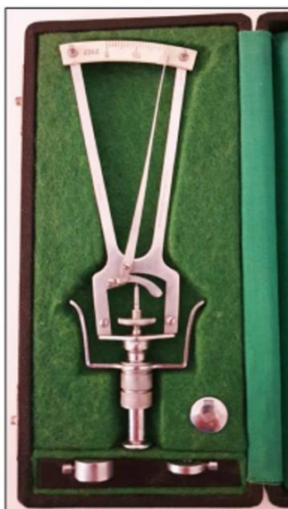
Figure 1. Schiøtz tonometer with different weights.
