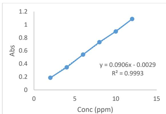
Figure 4a: Linearity curve for Formoterol fumarate dihydrate by zero order estimation.
