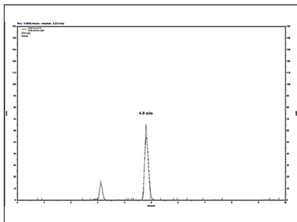
Figure 3: Chromatograph of Formoterol fumarate dihydrate showing retention time 4.8 min.
