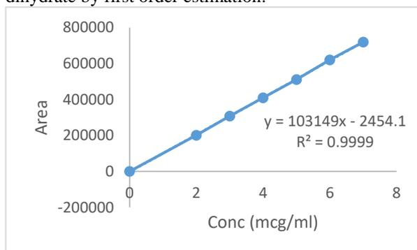
Figure 5: Linearity curve for Formoterol fumarate dihydrate by RP-HPLC.
