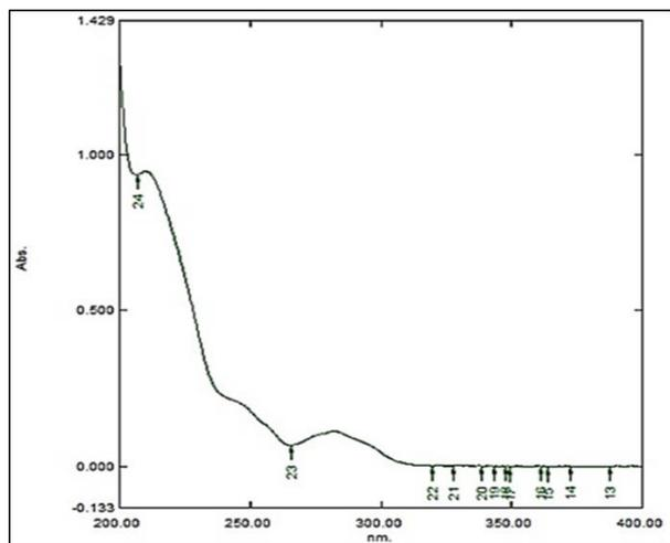
Figure 2: UV spectrum of Formoterol fumarate dihydrate showing  $\lambda$  max at 214 nm.
