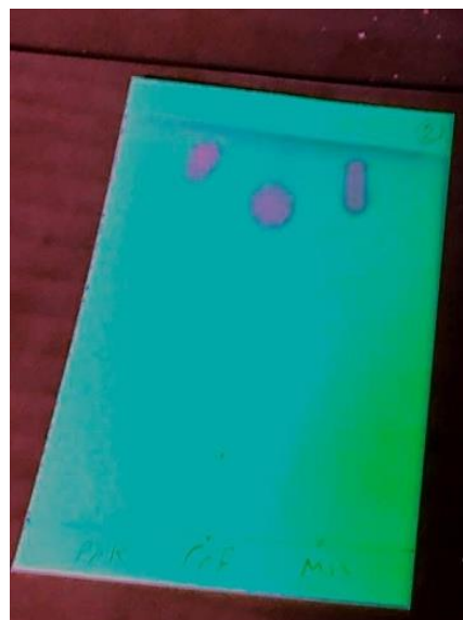
Figure 4: showing separation of paracetamol and caffeine by system B.
