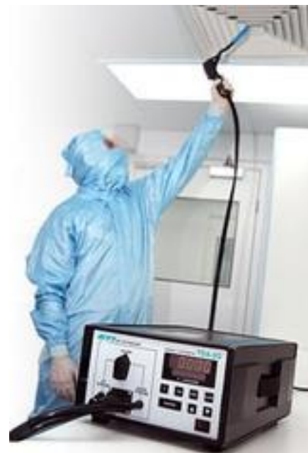
Figure 4: PAO Aerosol Generator and method of performing test [11]
